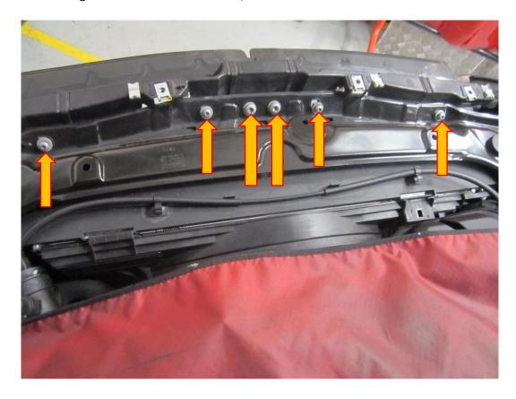
10. The last part of the slam panel to undo is the T30 Torx fastener which holds the slam panel to the head light. Remove both fasteners, one at each side of the vehicle. The slam panel will now lift out of the engine bay, pull it upwards and angle outwards to remove it from the vehicle.
