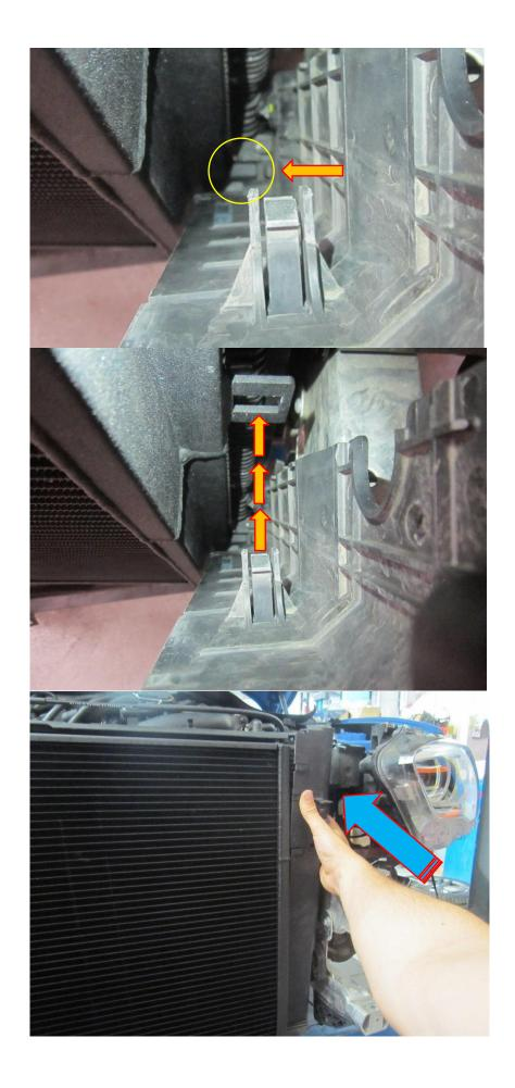
25. Reposition the radiator assembly back on the mounting hook and secure in place by re fitting the two T27 Torx fasteners. At this stage you can re fill the coolant back into the charge cooler system. Forge Motorsport recommend using Genuine BMW coolant. Undo and remove the bleed screw then fill the system with a
