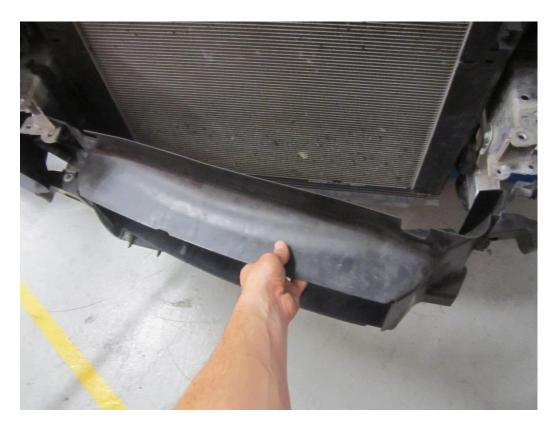
**16**. The lower bumper support is secured in place with two E11 fasteners, undo both fasteners and remove the support from the vehicle.
