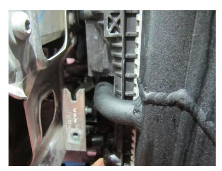
24. Make up the radiator frame by attaching the bottom panel to the side panels using the T27 fasteners removed earlier. Once the three parts are together position the pegs at the bottom of the Forge radiator with the mounting point at the bottom of the frame. Now push fit both sides of the frame and locate the fastening clip into its locating point on the Forge radiator. Re fit the two T27 Torx fasteners that attach the top part of the radiator frame to the frame sides.
