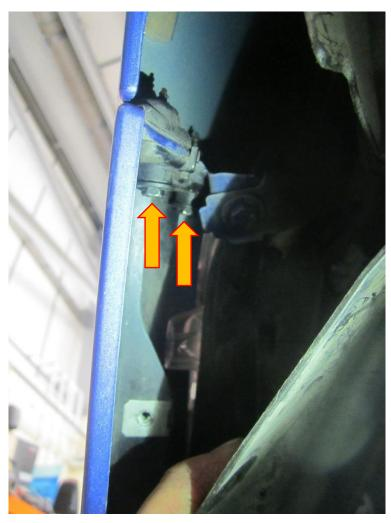
6. Unclip the loom to the temperature sensor that is located on the nearside of the inner bumper.
