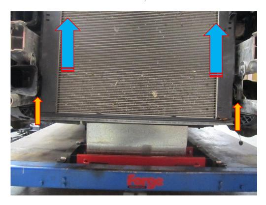
19. The two sides to the radiator frame are attached to the charge cooler radiator, these will simply pull away with a sharp tug.
