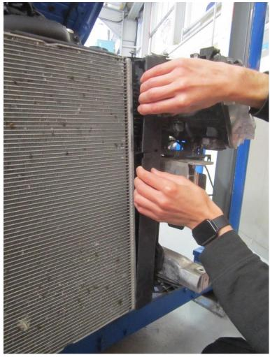
**20**. Remove the offside brake ducting, It is held in place with two plastic fasteners. Remove both fasteners to free the ducting from the vehicle.
