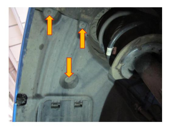
5. Now with the splash guard removed from the vehicle you will see the two 8mm fasteners that are attaching the top corner of the bumper to the wings, these both need to be removed on opposite sides of the vehicle.
