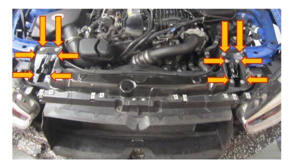
9. The next part of the slam panel removal is to locate the four T30 Torx and two T45 Torx fasteners which will all need removing with the relevant Torx driver/socket and rachet.
