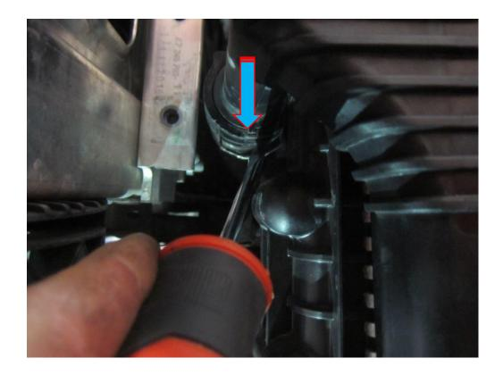
23. install your new Forge Motorsport FMCCRAD11 where the OE radiator fitted and re connect the coolant hoses, this should have a positive click when housed correctly.
