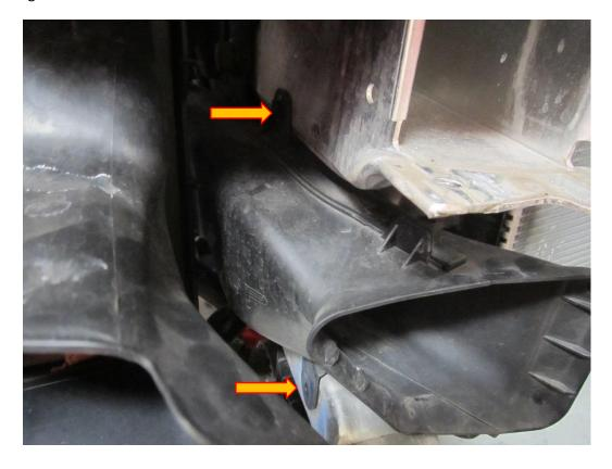
**21.** Place a drain pan or bucket under the offside hose going to the OE charge cooler in order to catch the coolant.
