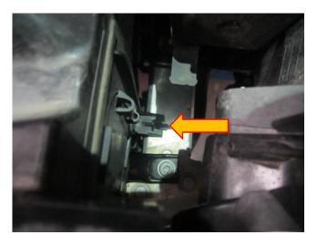
13. The support brace above the crash bar needs to be removed, it is held in place with two T45 Torx fasteners, the bar will now be free from the vehicle. Next remove the four 13mm fasteners which attach the crash bar to the vehicle, once removed the crash bar can be removed from the vehicle.
