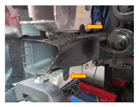
15. With the brake duct removed the lower air duct will now pull away from the vehicle.
