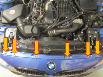
8. With the bumper off the vehicle you will need to remove the four T40 Torx fasteners located at the top of the slam panel, then remove the eight T30 Torx fasteners which secure the bonnet catches. Push the bonnet catches through the gap in the slam panel to make the removal of the panel easier.
